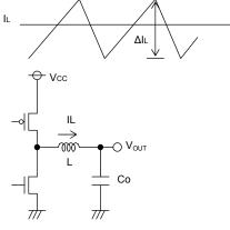
The inductance significantly depends on output ripple current. As seen in the equation (1), the ripple current decreases as the inductor and/or switching frequency increases.
