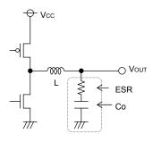
Output capacitor should be selected with the consideration on the stability region and the equivalent series resistance required to smooth ripple voltage.
