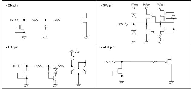
Fig.36 I/O equivalent circuit
