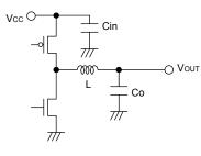
Fig.30 Input capacitor
