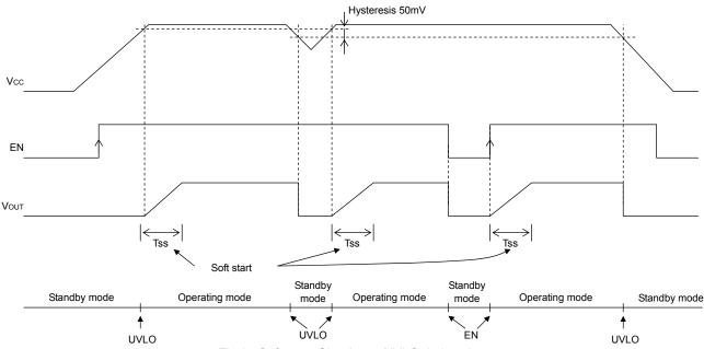
Fig.25 Soft start, Shutdown, UVLO timing chart
