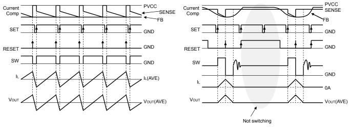
Fig.23 PWM switching timing chart
